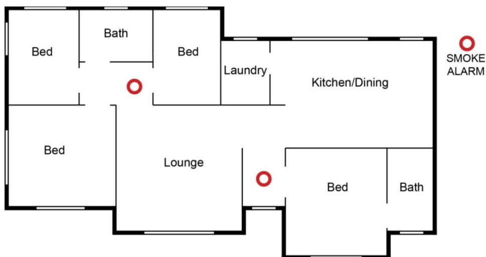
Figure 6 Smoke alarm placement in Class 1a, 2, 3 and 4 dwellings - ungrouped bedrooms
