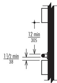
**Fig. 12f** Protruding Objects Mounted Near Grab Bars.
