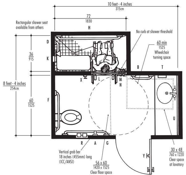
**Fig. 32** Bathroom with Combination Tub/Shower Unit and Portable Seat.
