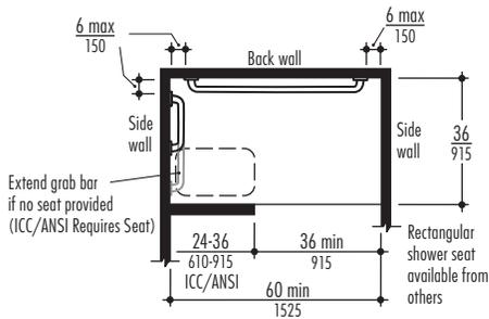
**Fig. 24c** Alternate Roll-In Type Shower Compartment (with seat).
