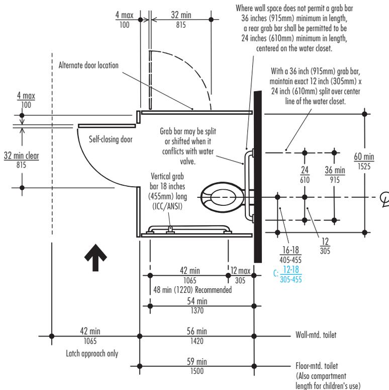
Fig. 9 Large Wheelchair Accessible Toilet Compartment.
