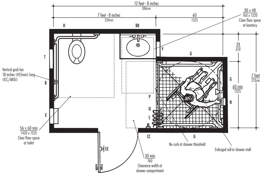
**Fig. 30** Bathroom with Roll-in Shower Compartment.
