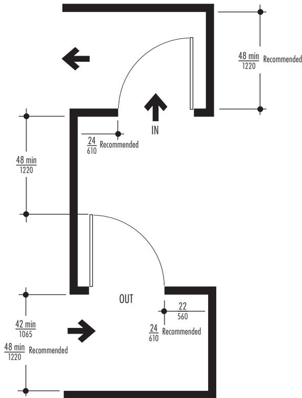
Fig. 3b Opposing Doors. (Door has closer and no latch)
