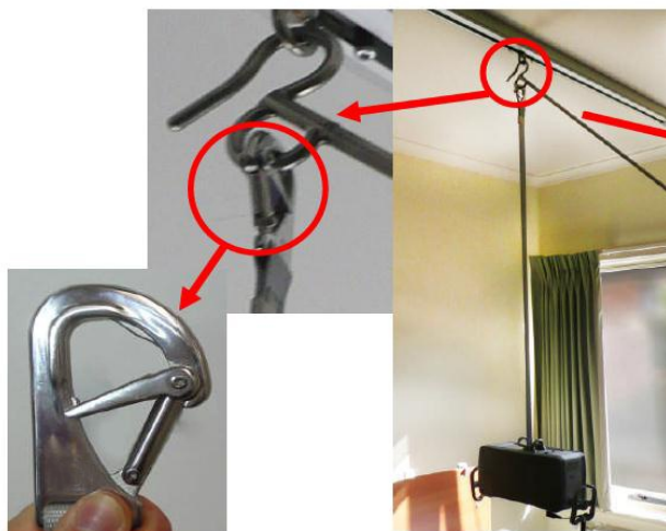
Figure 1: Patient handling ceiling hoist that uses a latching hook and wand system.
