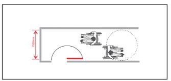
A corridor needs to be 1500mm wide to allow wheelchairs to pass each other and to allow a 360 degree turn.
