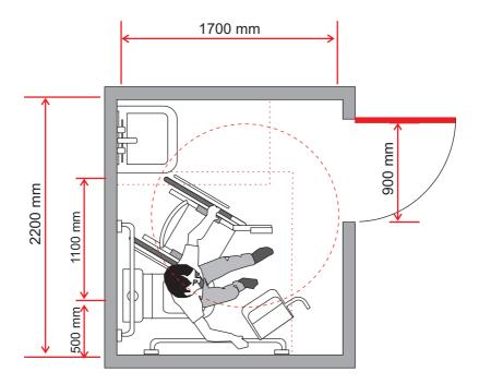
Design layout for a toilet showing a wheelchair user performing a lateral transfer. This bathroom layout does not offer the opportunity for a front transfer. Note the critical space between the exposed edge of the toilet and the wash hand basin, which allows the wheelchair to manoeuvre beside the toilet.
