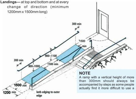
Ramp with gentle 1:15 slope. Note landings at top, bottom and mid-way. Observe that the top landing is measured from the top of the ramped surface to the edge of the door opening circle. Note also railings on both sides as well as curb on exposed edge of ramp (inset). Curbs help prevent people and mobility aids from falling off the ramp. Step access is also shown.
