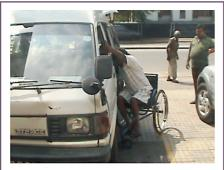
**Space required beside the vehicle** Additional space is required beside the vehicle so the person can safely move in and out of the vehicle with their equipment, as shown in this picture.
