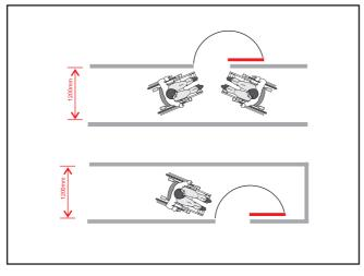
A corridor needs to be 1200mm wide to allow a wheelchair to make a 90 degree turn into a door when the door is 800mm wide
