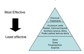
Figure 9: The effectiveness of different active ingredients found in surface coatings
