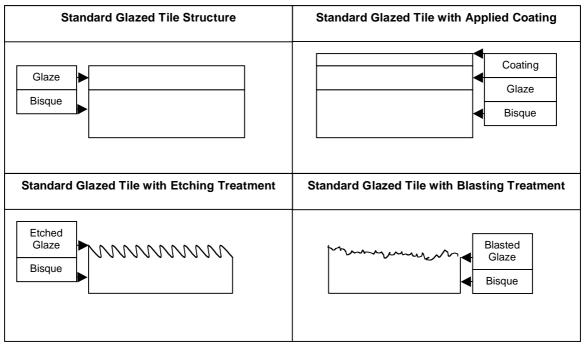
Figure 1: Interventions that increase the COF of a standard glazed tile.
